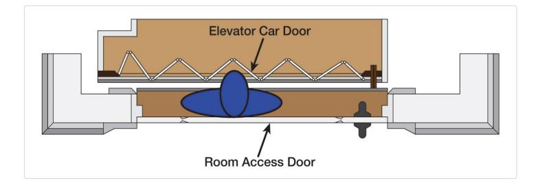
If the gap is too large, a small child can become entrapped between the room access door and the elevator car door.
